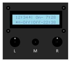
After two minutes the display turns off. Pressing the middle or right button, or turning the right button, turns the display back on. The **left button** is used to adjust the sensitivity to the light. Only turn it when the twilight is not detected properly.
